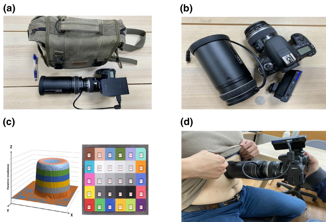
FIGURE 1 The highly accurate, portable, low-cost skin color image system. The system weighs 1.5 kg and is 30 cm in length and 13 cm in width. It composites three key elements: a sunlight light-emitting diode ring light, a dark room module, and a digital single-lens reflex camera (Canon DSLR, 77D) with a macro lens (EF-S, 60 mm). The plot of the standard color difference was derived from our previous conference paper. 10 The 1d) exhibits that applying the imaging system takes a leaning backward sitting subject's skin color image. (a) The small size of the developed image system (length/width: 30/13 cm). (b) The components of the developed image. (c) Standard color difference of the developed image system. (d) Taking skin color image by leaning backward sitting.
